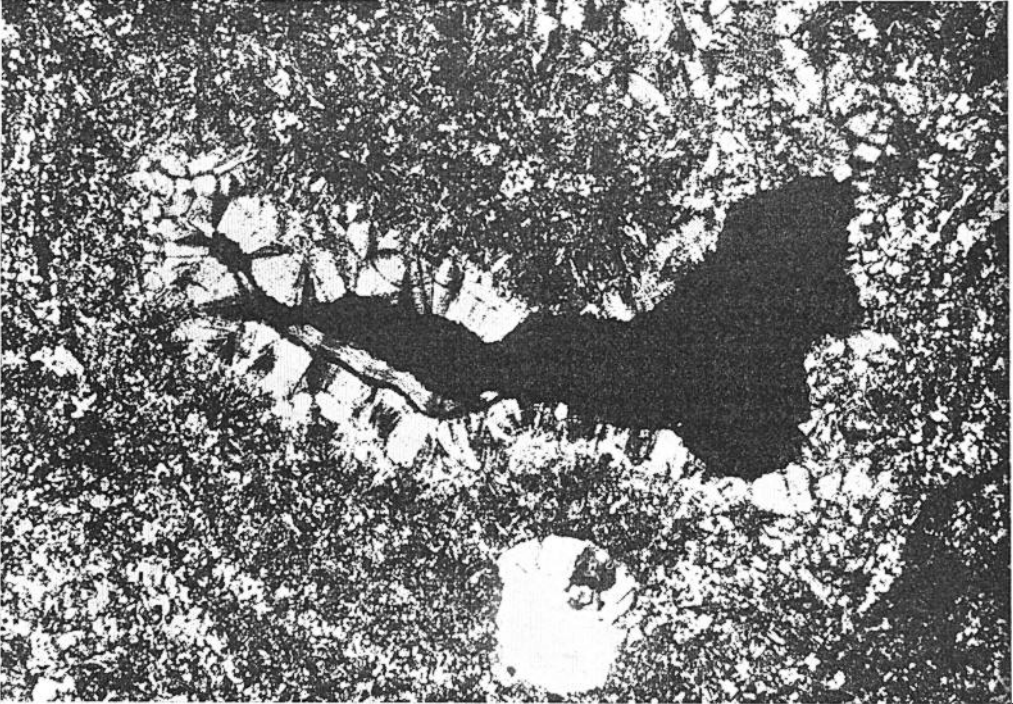
FIG. 36. Same, with nicols crossed, showing the radial fibrous structure of the lussatite.
