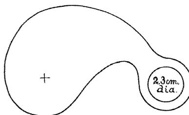
in diameter (a hair larger than the outside diameter of the standard eyepiece) is bored by means of an extension bit at one end of the screen. The distance from the center of this hole to the middle point of the broad wing of the screen is 8 cm. The extreme length and width of the screen is 12.5 cm. by 7.5 cm.
