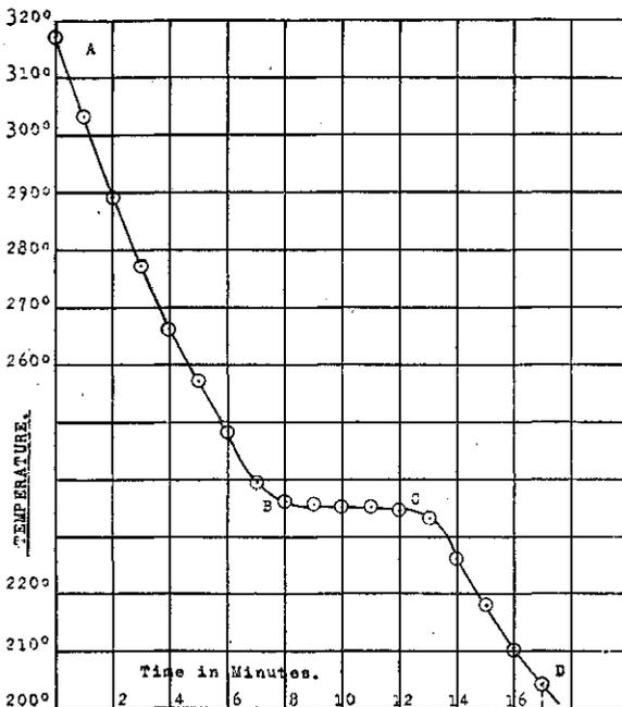
FIG. 2. SHOWING THE COOLING-CURVE FOR TIN.
