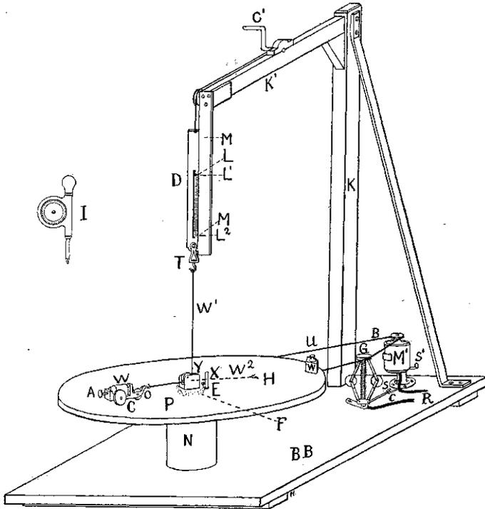
Apparatus consists mainly of wooden disk P about 2 ft. 6 in. in diameter, mounted on the base BB and rotated on ball bearings F; an inverted L shaped arm K, 3 ft. long, placed so that the end of its arm comes directly over the disk. A three wheel car C, on the disk receives the weight W. A wire W' passes from the car through the pulley Y to the swivel T, which is connected to the dynamometer D, that being suspended by a rawhide cord K'. The other end of K' is made fast to crank C. The disk is
