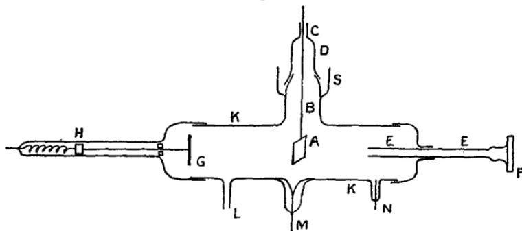
These improvements consisted in making the tube KK (fig. 1) wider (7 cm. diameter), the inlet for the light narrower, and the platinum electrode G larger. As before
