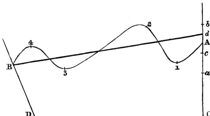
the line required, as may easily be seen by comparing the portions given and taken by the respective fields. This line would only divide the fields perfectly accurately as before, if A 1 2, 2 3 4, &c., were rectilinear angles; but it is the nearest approximation possible, and the one always used.
