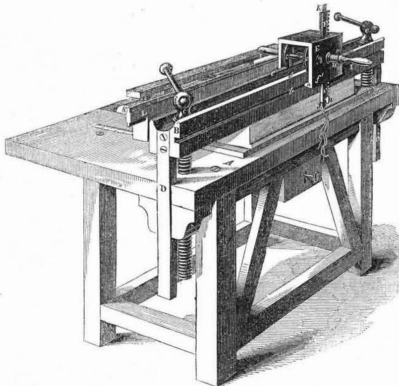
The annexed engraving is a perspective view of a machine for cutting paper, pasteboard, &c., for which a patent was granted on the 19th of last July (1853) to H. J. Oerter, of Bethlehem, Pa. The nature of the improvement consists in having an adjustable
