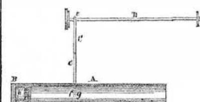
the clamps are provided with points, f, f. The rod, D, has a screw thread cut upon it, at one end, which screw-thread passes into the centre of the screw, a, as the rod, D, is turned, and the rod and clamps are thereby secured within the case, A. In order to detect counterfeit coin, the gauge box, B, is withdrawn from the case, A. If the coin will pass snug-
